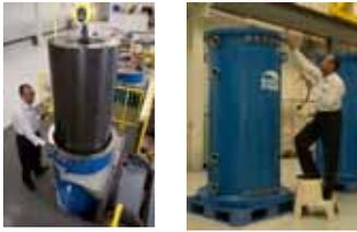
Volant fibre carbone 1 tonne
